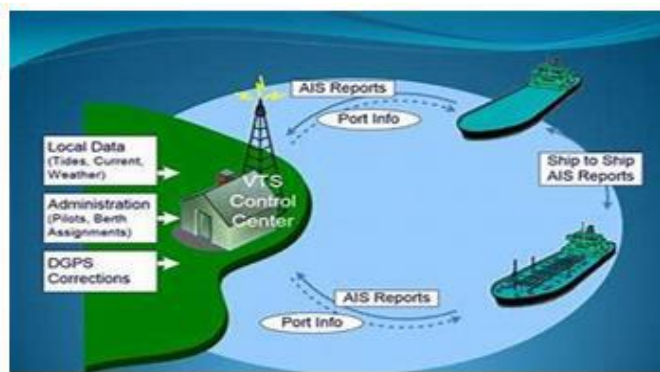
Figure 2: Illustrates the Mechanism of Data Exchange in the AIS System between Ships and Ports
